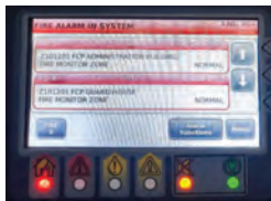
Fig.4 Fire alarm local control panel and fire alarm center control panel in control room show alarm zone admin building
